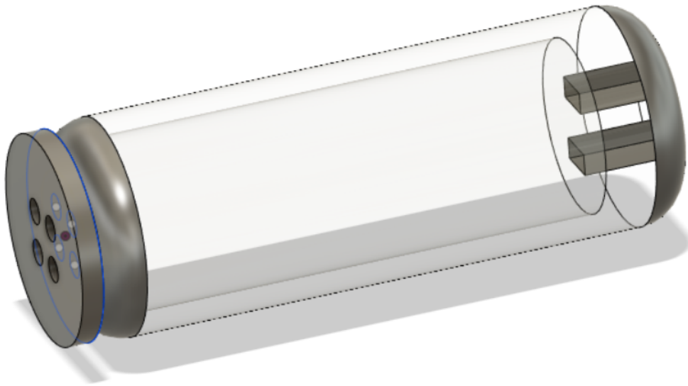
Figure 1 illustrates diagram of an embodiment of the device as a whole, as well as the holes strategically placed on the top of the device to allow for gas to escape and the two holes for oxygen and nitrogen input.
